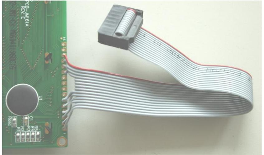
Note that the red wire is connected to pin J2.1
