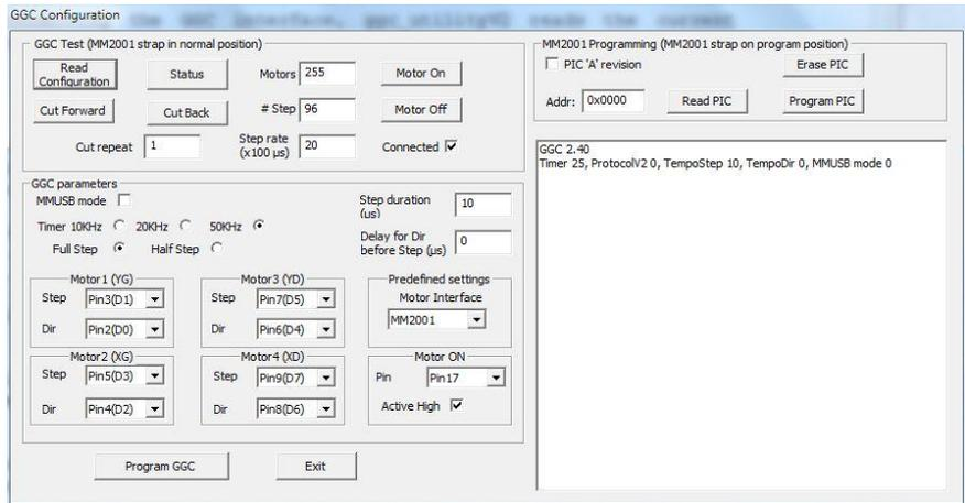
The GGC interface is shipped configured in MMUSB mode. If you want to switch to the GGC mode, you must uncheck the '**MMUSB mode**' box. Then you can modify the appropriate internal timer frequency and motor timing parameters. Additionally, to avoid rewiring motor cables, you can simply reconfigure the motor outputs. Finally, you can set the pinout for the "Motor On" signal (1 or 17) and also the active state ("Low" or "High").
