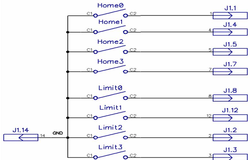
The Home switches and Limit switches are used to prevent accidental over-run beyond the physical limits of the X and Y axes. The Home and Limit switch options are only functioning when running the GMFC EXPert software. They do not function under any other version of GMFC. Home and Limit Switches must be of type "Normally Open".
